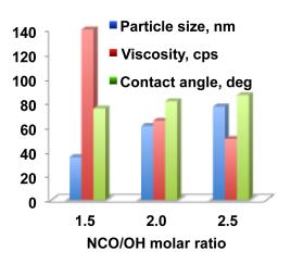
Figure 2 – The effect of NCO/OH ratio on particle size, viscosity and contact angle of PUD
