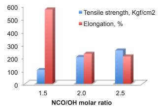
**Figure 3** – The effect of NCO/OH molar ration on the tensile strength and elongation of PUD.
