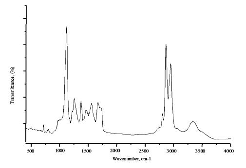
Figure 1 - FTIR of polyurethane dispersion.
