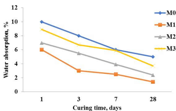
Figure 4 – The effect of St/BuA lattices on the water absorption of mortar
