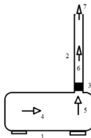
**Figure 5** – Technological scheme of the installation and the functional principle of the catalyst in the furnace of oil heating: 1 – Furnace of oil heating, 2 – flue, 3 – catalytic neutralizer, 4,5 – stream of waste gases ( $\text{CO}$ ,  $\text{CH}_x$ ,  $\text{NO}_x$ ) before the catalyst, 6,7 – the flow of gases after the catalyst ( $\text{H}_2\text{O}$ ,  $\text{CO}_2$ ,  $\text{N}_2$ ).
