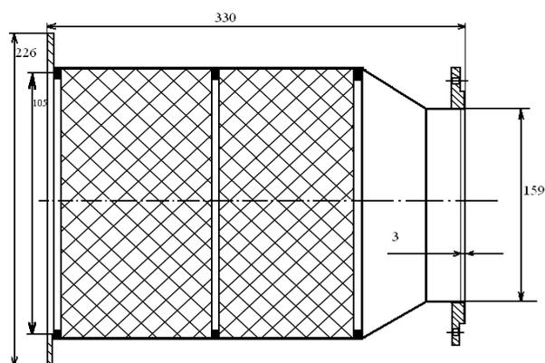
**Figure 4** – Dimensions and the scheme of disposition of the catalytic neutralizer in the case
