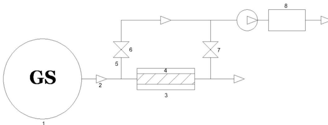
1 – Diesel generator; 2 – exhaust pipe; 3 – catalytic reactor; 4 – catalyst sample; 5 – gas operated probe; 6, 7 – sampling valves before and after the catalyst; 8 – a gas analyzer.
