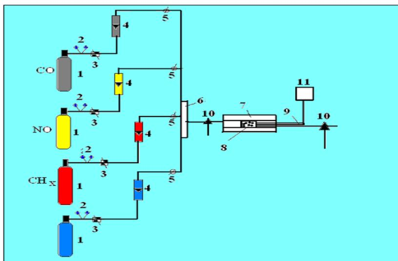
**Figure 1** – Scheme of the flowing installation: 1- A gas bag; 2-Manometer; 3-Ventile of thin regulation; 4-Rotameter; 5-Crane; 6-Mixer; 7-Heating system; 8-Catalyst; 9-Thermocouple; 10-Selection of tests before and after the catalyst; 11 – Temperature regulator.
