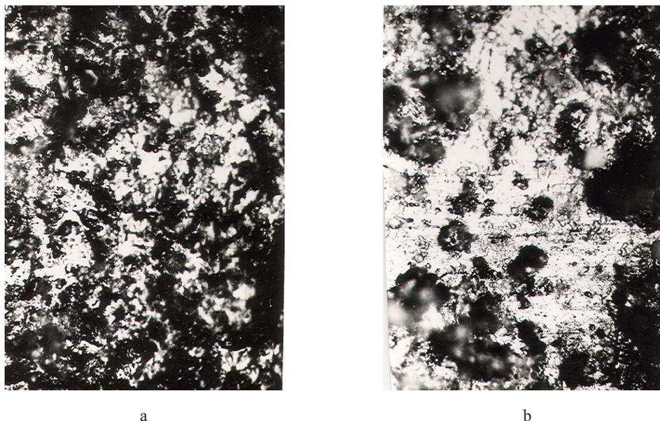
Figure 6 – The nanosized particles (300, 000 magnification) : a – Pt, b – Pd
