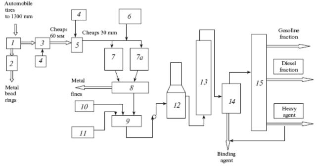
Figure 1 - Schematic diagram of the utilization of car and heavy-duty tires as chips: 1 sorting floor, 2 side strip remover, 3 cutter-type chipper, 4 electromagnetic apparatus, 5 hammer mill, 6 tank with a solvent spent oil, 7, 7a chip fluidization reactor, 8 magnetic separator, 9 mixer homogenizer, 10 tank with petroleum residue, 11 zeolite shale crushing and dispensing unit, 12 furnace, 13 thermolysis reactor, 14 separator, and 15 rectification column [From literature 4].
