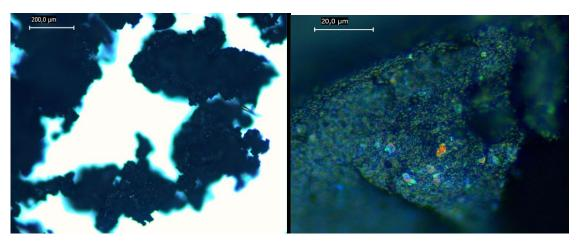
Figure 2 - Optical microscope images of rubber crumb with particle size less than 0,6 mm (activated)
