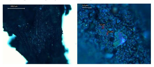
Figure 3 - Optical microscope images of rubber crumb with particle size 0,6-1,0 mm (no activated)
