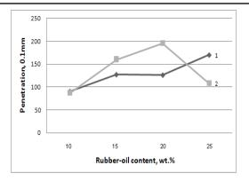
1 – activated rubber modified bitumen (R:O=1:1)
