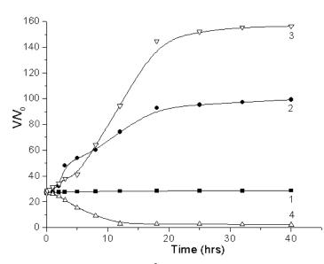
T = 20<sup>0</sup>C, [HEA]:[HEMA] = 71.7:28.3 mol%, in [SDS],  $10^{-3}$ mol/L: 1 (sample V1) – 5; 2 ( sample V2) – 16; in [CPB],  $10^{-4}$ mol/L: 3 (sample V3) – 1; 4 (sample V4) – 10.
