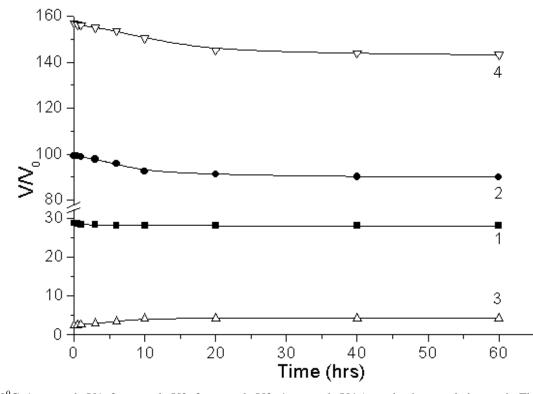
$T = 20^{\circ}C$ , 1 – sample V1; 2 – sample V2; 3 – sample V3; 4 – sample V4 (sample characteristics see in Fig. 3). **Figure 4** - Kinetics of swelling ratio changes of HEA-HEMA-surfactant complexes after interaction with surfactants solutions.
