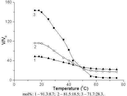
Figure 6 – Dependence of swelling ratio of HEA-HEMA-CPB complexes on the temperature in aqueous solutions. Content of HEA-HEMA copolymers used: [HEA]:[HEMA].
