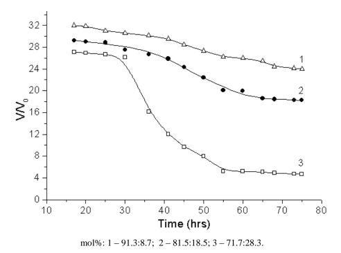
**Figure 2** – Dependence of swelling ratio of HEA-HEMA hydrogels on the temperature in aqueous solutions. [HEA]:[HEMA].,
