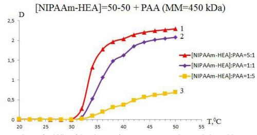
**Figure 6** — Dependence of turbidity of the mixtures of NIPAAm-HEA copolymer solutions with PAA on temperature. Note: [NIPAAm-co-HEA]=[PAA]=0,1 g/dL; IMM[NIPAAm-HEA]=50-50 mol %; MM(PAA)=450000 Da; [NIPAAm-co-HEA]:PAA=5:1 (1); 1:1 (2); 1:5 (3)
