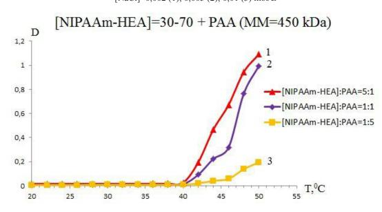
**Figure 5** — Dependence of turbidity of the mixtures of NIPAAm-HEA copolymer solutions with PAA on temperature. Note: [NIPAAm-co-HEA]=[PAA]=0,1 g/dL; IMM[NIPAAm-HEA]=30-70 mol %; MM(PAA)=450000 Da; [NIPAAm-co-HEA]:PAA=5:1 (1); 1:1 (2); 1:5 (3).
