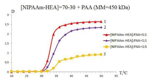
**Figure 7** — Dependence of turbidity of the mixtures of NIPAAm-HEA copolymer solutions with PAA on temperature. Note: [NIPAAm-co-HEA]=[PAA]=0,1 g/dL; IMM[NIPAAm-HEA]=70-30 mol %; MM(PAA)=450000 Da; [NIPAAm-co-HEA]:PAA=5:1 (1); 1:1 (2); 1:5 (3)
