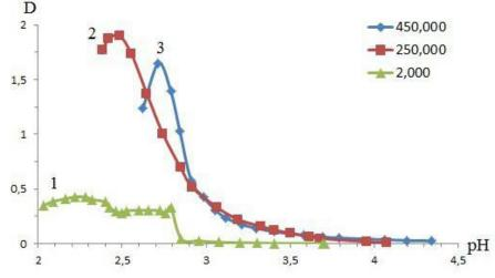
**Figure 2** — Dependence of optical density of the mixtures of NIPAAm-co-HEA copolymer solutions with PAA of different molecular weight on pH.
