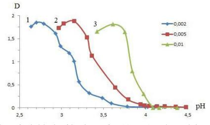
**Figure 4** — Dependence of optical density of the mixtures of NIPAAm-HEA copolymer solutions with PAA on pH at various ionic strength of medium.
