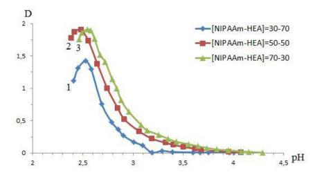
Figure 3 — Dependence of optical density of the mixtures of NIPAAm-HEA copolymer solutions of various compositions with PAA on pH.
