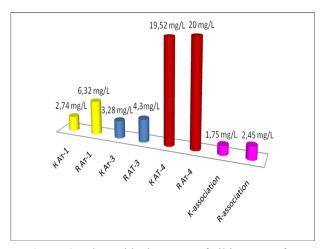
Figure 4 - The residual amount of oil in water after treatment.
