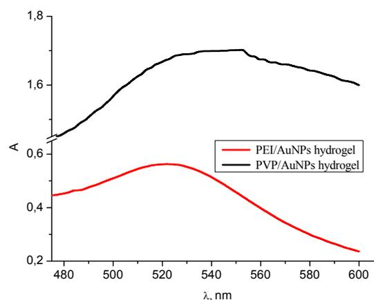
**Figure 3** – UV-Vis spectra of AuNPs hydrogels
