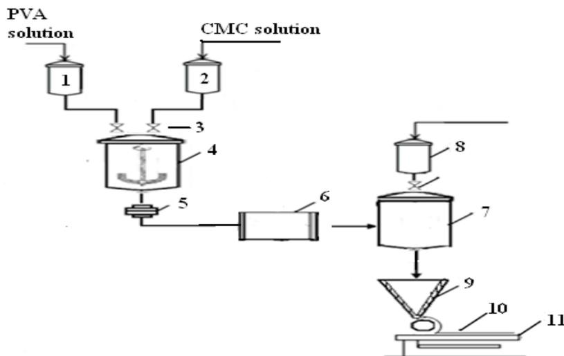
1 – bunker of PVA solution; 2 – bunker of CMC solution; 3 – dosing devices; 4 – reactor for the mixing of initial components; 5 – filter; 6 – electron accelerator ELV-4; 7 – mixer for introducing of the drug into the hydrogel; 8 – storage tank of drug; 9 – фильера; 10 – cutting; 11 – packaging.
