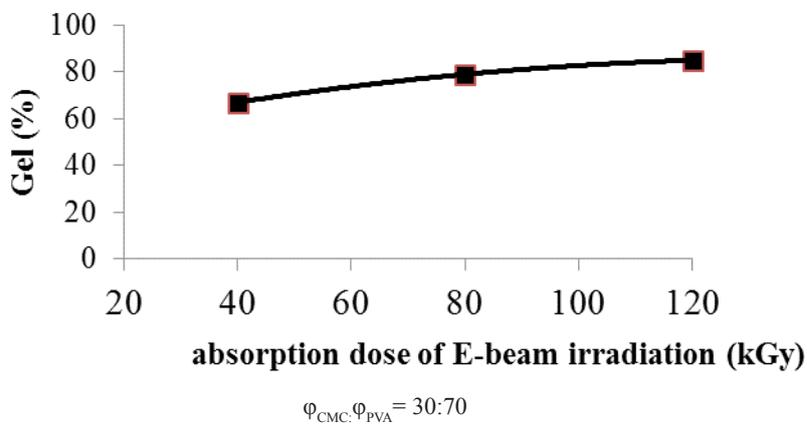
Figure 2 – Gel fraction of crosslinked CMC/PVA hydrogels at various absorption dose of E-beam irradiation (kGy) .
