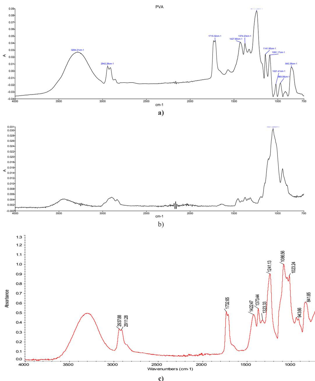
Figure 3 – FTIR spectra of PVA (a); CMC (b) and composite material based on CMC/PVA (c)
