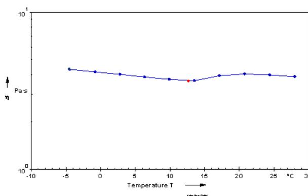
**Figure 10** – Effect of temperature on the viscosity of a hydrogel ointment based on carbopol with 1%  $\alpha$ -lipoic acid
