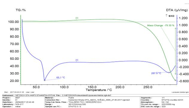
**Figure 7** – Differential-thermal analysis curves (DTA) of the substance of lipoic acid
