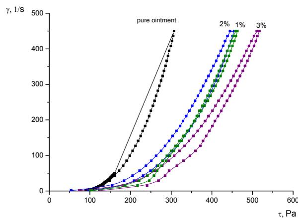
Figure 9 – Rheogram "Hysteresis loop" of hydrogel ointments based on carbopol with different concentrations of  $\alpha$ -lipoic acid
