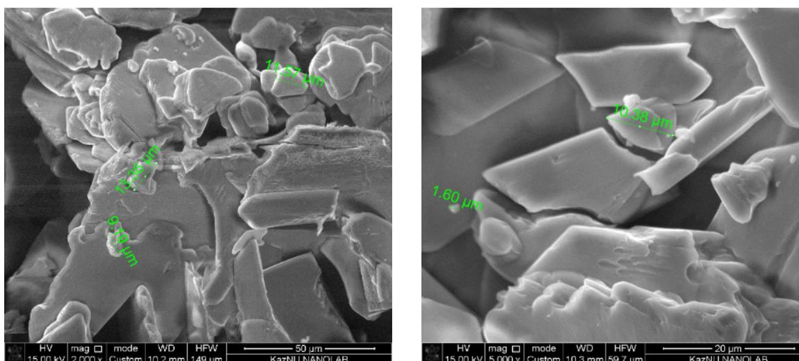
**Figure 4** – Raster electron microscopy of  $\alpha$ -lipoic acid substance at magnification 2000 (left) and 5000 (right)
