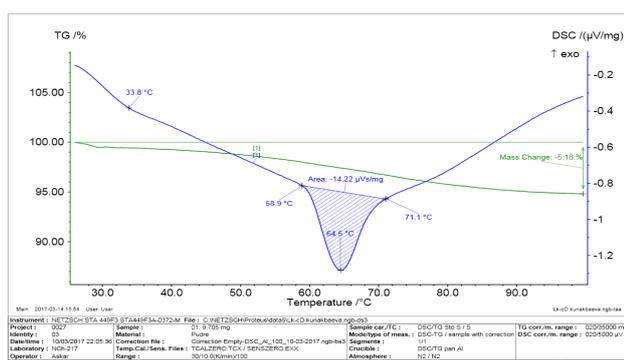
Figure 2 – TGA-DSC analysis of the inclusion complex of GP- $\beta$ -CD and ALA obtained by grinding
