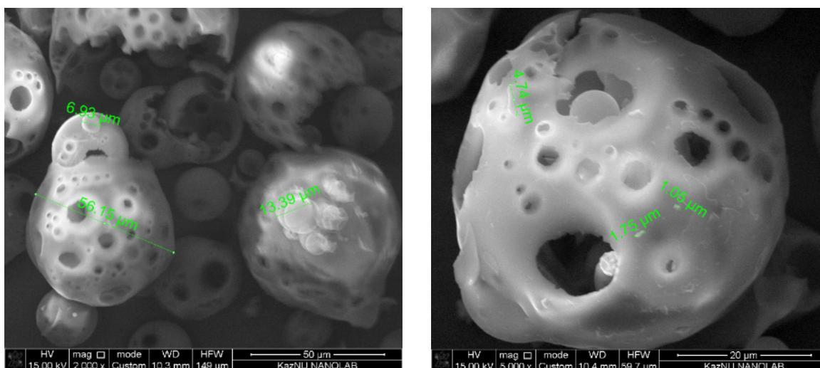
**Figure 3** – Scanning electron microscopy of the substance hydroxypropyl- $\beta$ -cyclodextrin at magnification 2000 (left) and 5000 (right)
