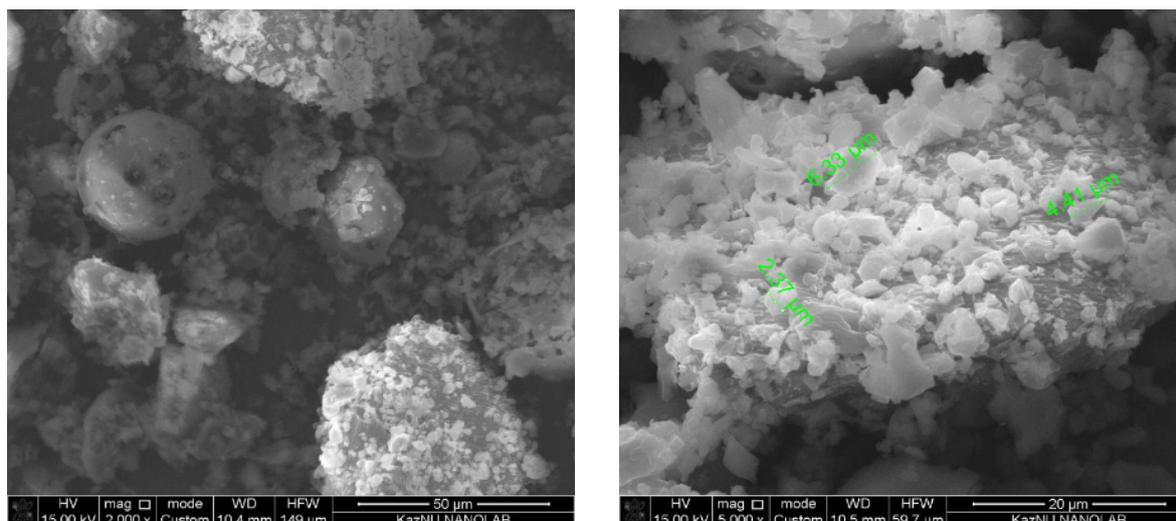
**Figure 5** – Raster electron microscopy of the ALA-HP-β-CD complex obtained by grinding at magnification 2000 (left) and 5000 (right)
