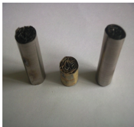
Figure 1 – the laboratory samples of neutralizers on metal blocks
