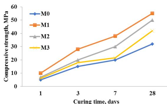
Figure 3 – The effect of St/BuA lattices on the compressive strength of mortar
