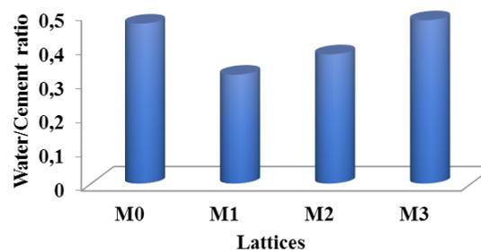
Figure 1 – The effect of St/BuA lattices on the water/cement ratio of mortar
