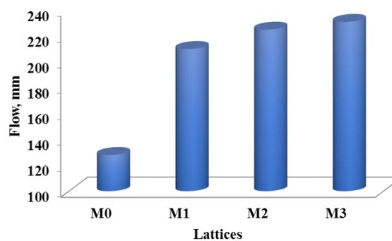
Figure 2 – The effect of St/BuA lattices on the workability of mortar
