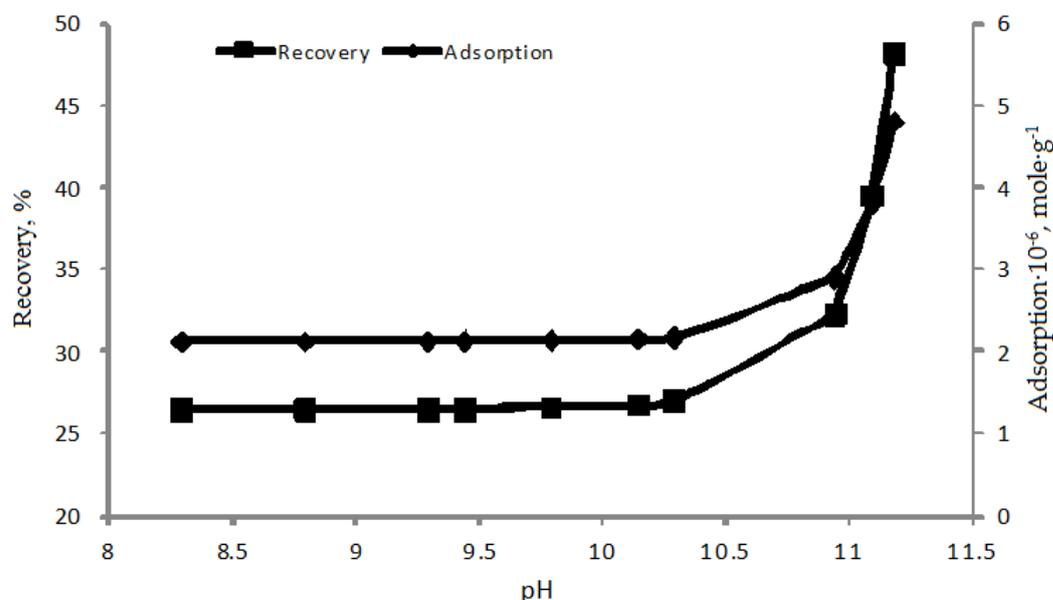
**Figure 1** - The effect of pH on copper recovery and the adsorption of sodium diisopropyldithiophosphate ( $C=4.25 \cdot 10^{-5}$  mole $\cdot$ L $^{-1}$ ) on copper sulfide ore
