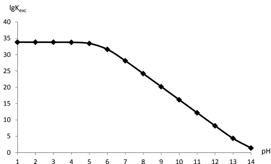
**Figure 2** - The effect of pH on the exchange constant of hydroxide-ions on diisopropyldithiophosphate ions in the composition of a poorly soluble compound
