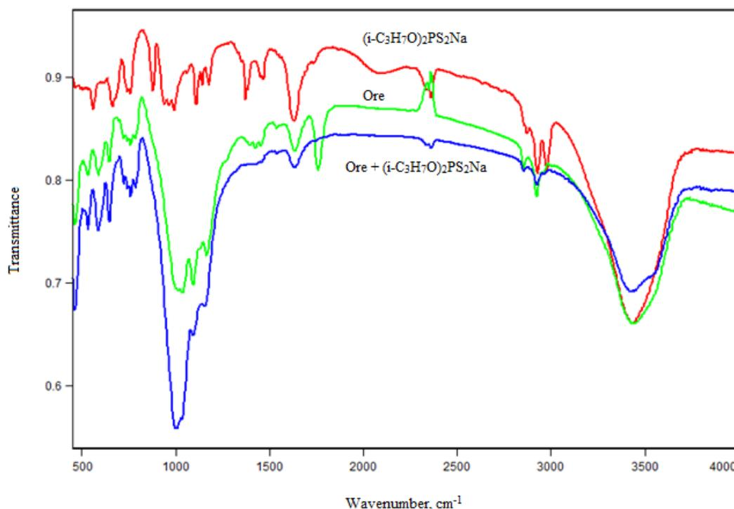
**Figure 5** – FT-IR spectra of collector, sulfide copper ore and sulfide copper ore treated with collector after treatment
