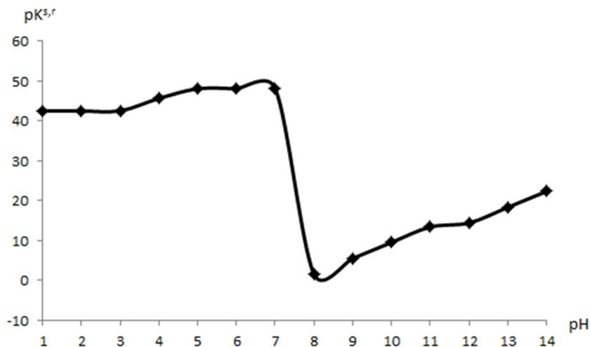
**Figure 3** – Dependence of the real solubility constant ( $pK^{S,r}$ ) of chalcocite in the presence of a flotation agent ( $C=4.25 \cdot 10^{-5}$  mole  $\cdot$  L $^{-1}$ ) on the pH of the mineral suspension
