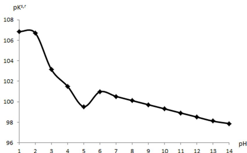
**Figure 4** – Dependence of the real solubility constant ( $pK^{s,r}$ ) of bornite in the presence of a flotation agent ( $C=4.25 \cdot 10^{-5}$  mole $\cdot$ L $^{-1}$ ) on the pH of the mineral suspension
