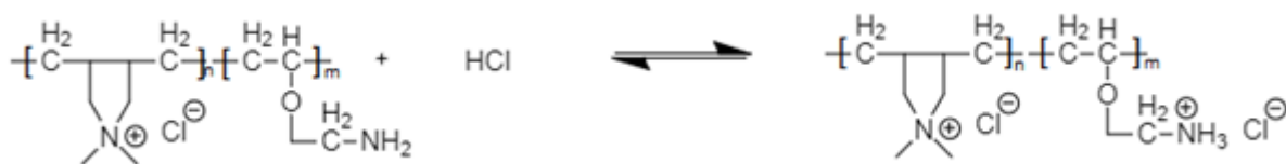
Scheme 2 – Interaction of amine group of the copolymer with hydrochloric acid
