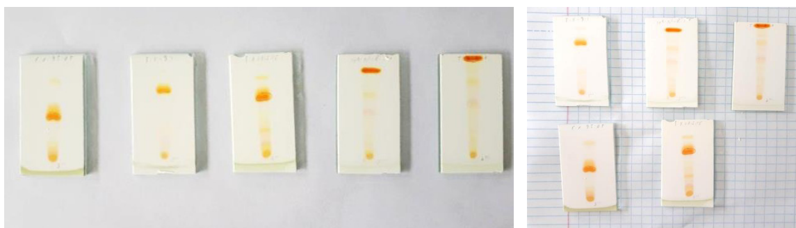
Figure 2 – Analysis of carotenoid concentrate from tomato mass by thin layer chromatography
