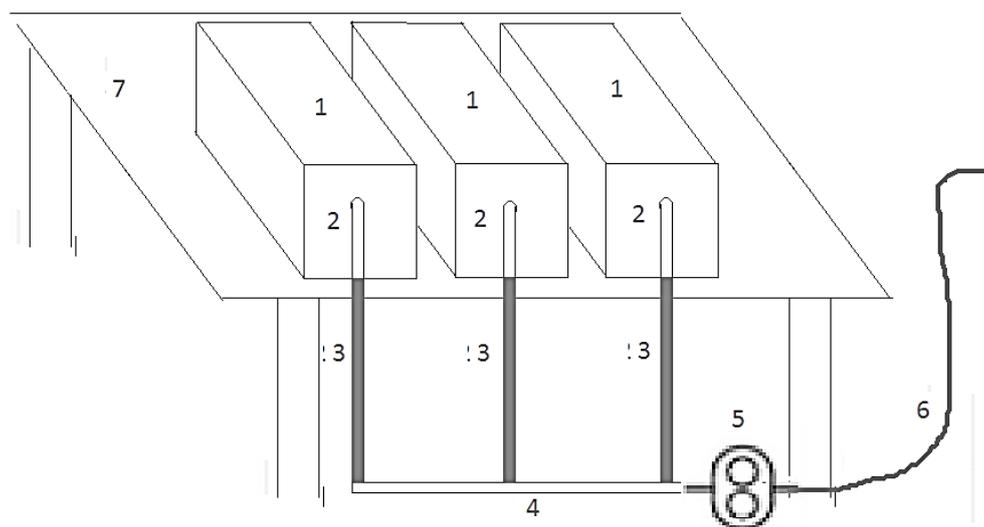
**Figure 1** – System for collection of volatile compounds excreted from Colorado potato beetle.
