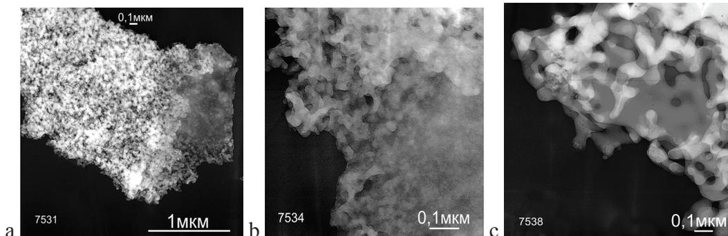
**Figure 1** – Electron micrograph of the surface of particles samples carbonized at 700-850°C
