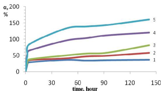
**Figure 1** – Kinetics of swelling of the hydrogel containing 5% concentration in water and saline [NaCl], % = 0,45 (2), 0,9 (3) 1,8 (4) 2,7 (5). In water (1)
