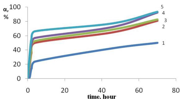
**Figure 2** – Kinetics of swelling of the hydrogel containing 7% concentration in water and saline [NaCl], % = 0,45 (2), 0,9 (3) 1,8 (4) 2,7 (5). In water (1)
