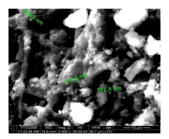
Figure 3 – Electron microscopic picture of Kiyakty deposit coal before mechanical activation.
