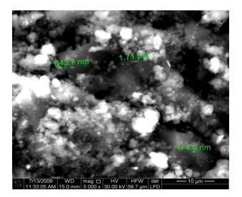
Figure 4 – Electron microscopic picture of Kiyakty deposit coal after mechanical activation.
