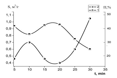
**Figure 2** – The change of specific surface S of milled coals (1) and porosity of coal (2) depending on the time of treatment.
