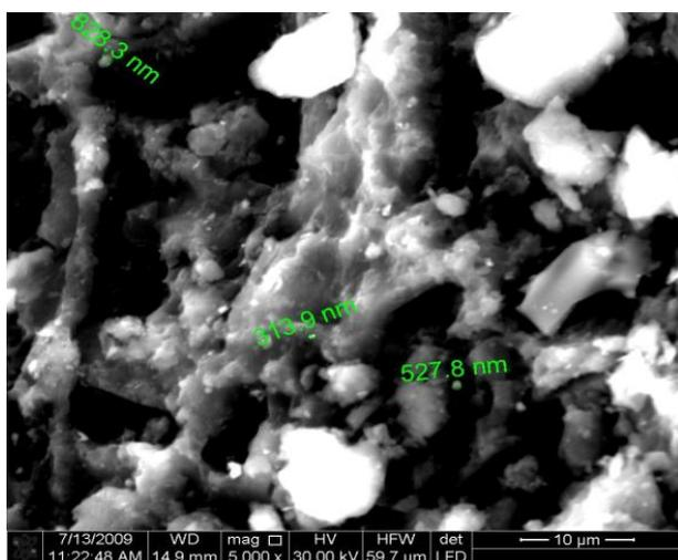
**Figure 3** – Electron microscopic picture of Kiyakti deposit coal before mechanical activation.
