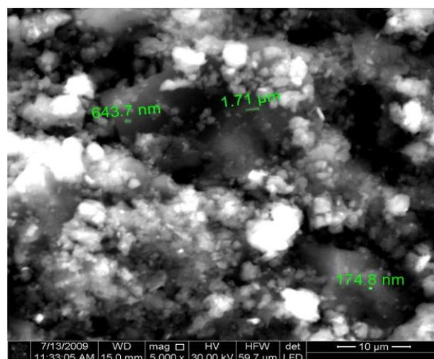
**Figure 4** – Electron microscopic picture of Kiyakti deposit coal after mechanical activation.
