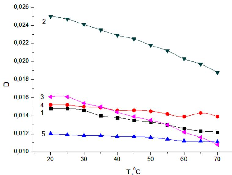
**Figure 3** – Temperature dependence of the optical density of aqueous solutions of [AA]: [MA] = 50:50, copolymer and PAA.
