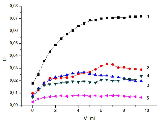
**Figure 1** - The turbidimetric titration curves of solutions of PAA with solutions AA-MA.
