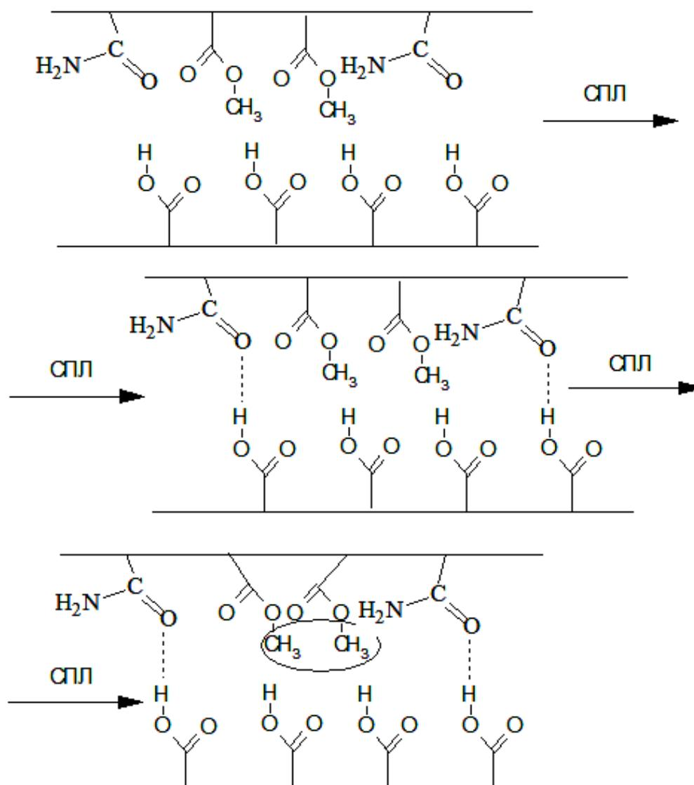
with PAA is carried by hydrogen bonds to form a hydrophilic associates, which reduces thermosensitivity.
