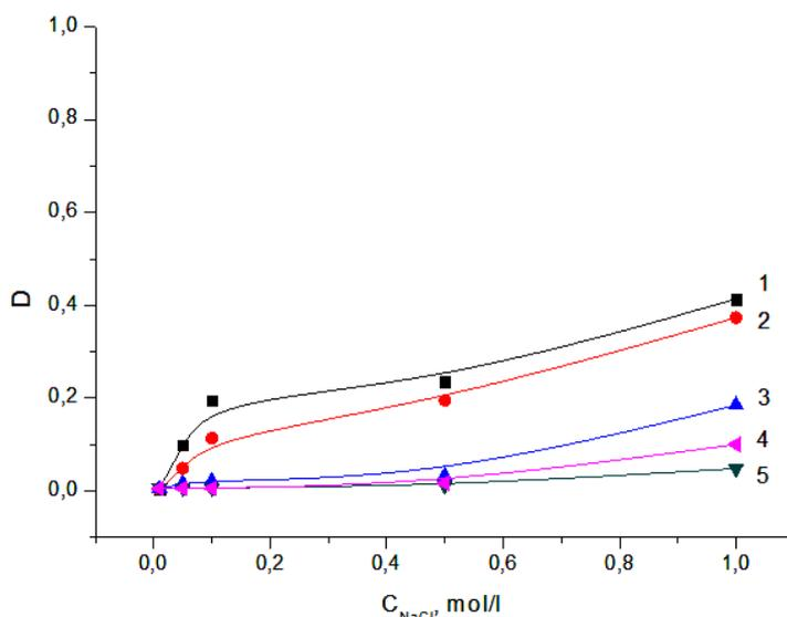
**Figure 4** - Influence of NaCl concentration on optical density of the copolymer aqueous solutions with PAA.
