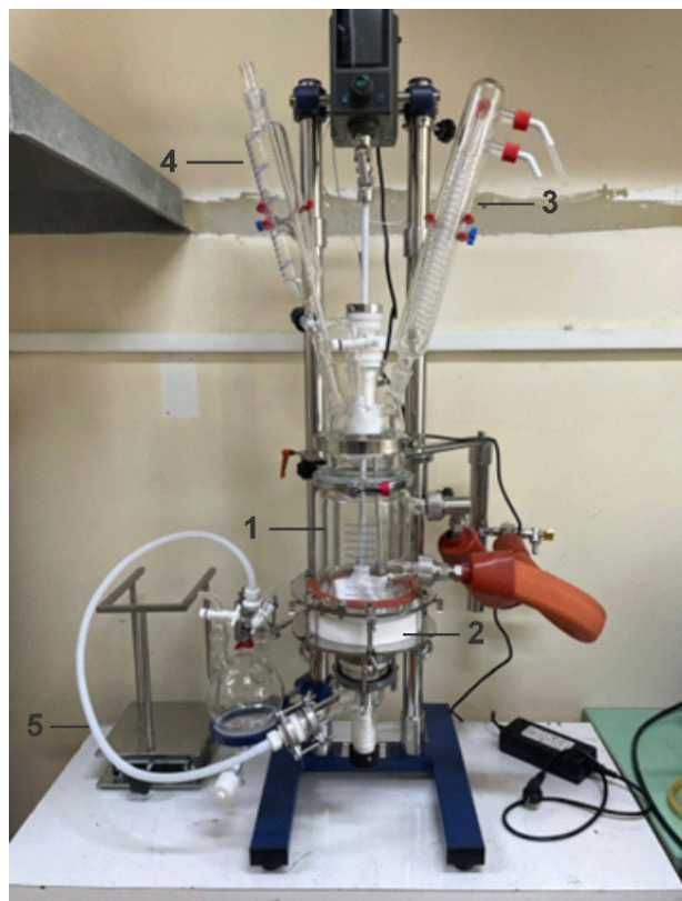
Figure 2 – Laboratory installation for obtaining magnesium sulfate solution: 1 – reactor, 2 – filter, 3 – thermometer, 4 – doser
