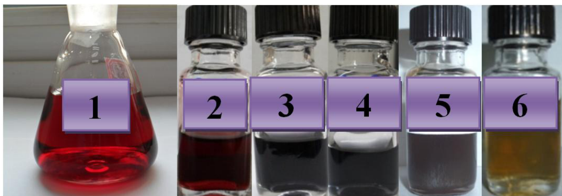
Figure 1 - Samples of AuNPs stabilized by sodium citrate (1), by PVP with M_n = 10 kD (2), 40 kD (3) and 350 kD (4), and AgNPs protected by PVP with M_n = 40 kD in DMF (5) and DMSO (6)
